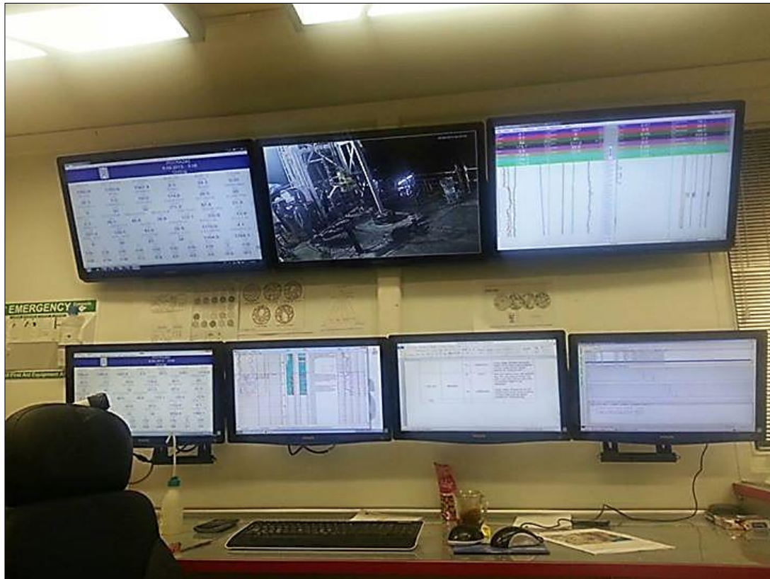
Figure 5.11. A view inside the mudlogging unit. All critical information about the drilling is collected in this unit and monitored instantly with many screens
