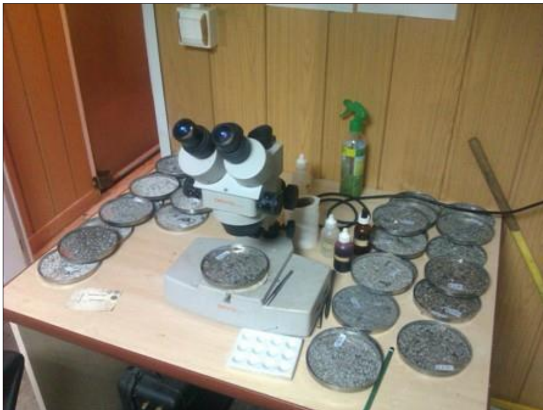
Figure 5.12. Rock fragments cut by drilling are examined under microscope. Lithologic well log is processed
